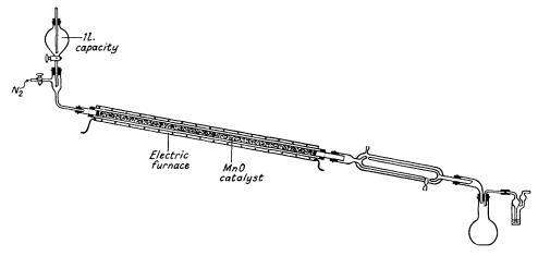
450° could be readily produced; *e.g.*, with a current of 1.0 amp. the temperature is 200°, and with 1.5 amps. it is 400°. The temperature was constant to within 1° up to 28 cm. from the ends of the iron tube and to within 5° 20 cm. from the ends.
